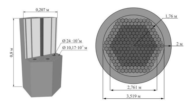
Fuel block and a cross-section of the thorium reactor core. Credit: Tomsk Polytechnic University
