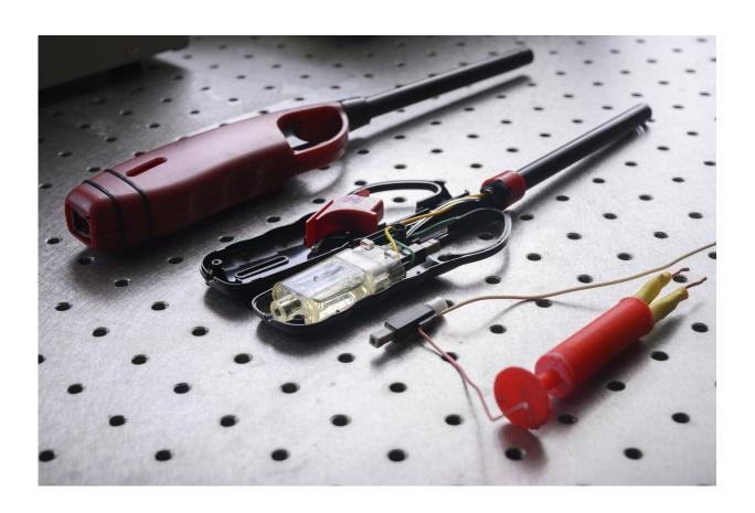
This image shows a common butane lighter (left) from which the researchers obtained a piezoelectric component used in the ElectroPen (right), an inexpensive electroporator which has a 3D-printed case. Credit: Christopher Moore, Georgia Tech
