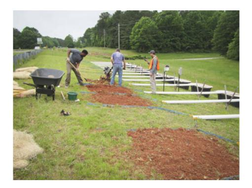
The researchers installed runoff collection systems to capture runoff from a highway. This way they could measure if their efforts were successful. Credit: Jamie Luther
