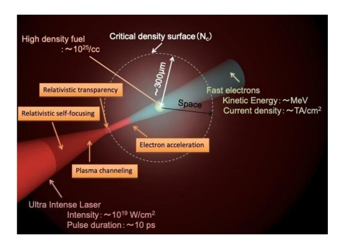
Fig.1 Schematic image of fast ignition laser fusion utilizing relativistic effects of ultra-intense laser light
