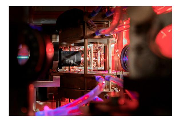
Picture of the single atom trap. In the ultra-high vacuum glass cell a single Rubidium atom is captured, which later will be entangled with a photon. Credit: C. Olesinski/LMU
