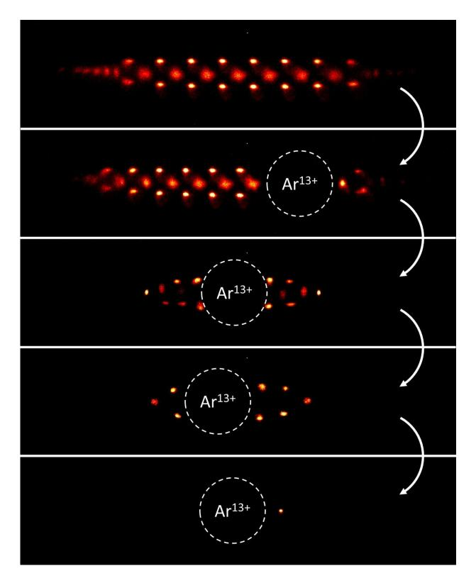
Implantation of the Ar13+ ion into the laser-cooled Be+ ion crystal and step-wise reduction to the quantum logic configuration of an ion pair. Credit: PTB
