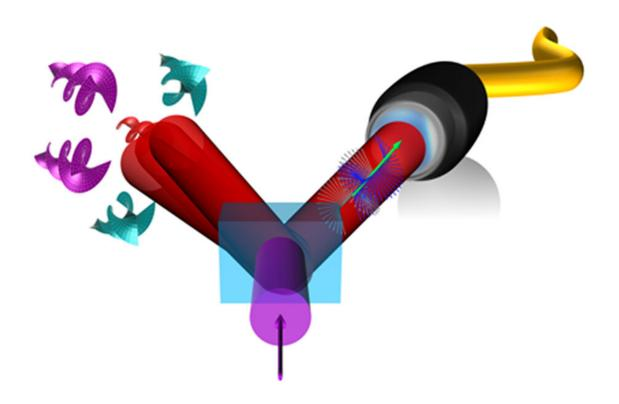
Two photons are entangled, one in polarization and the other in orbital angular momentum -- twisted light. By passing the polarization photon through the fiber and keeping the twisted light in air, multi-dimensional entanglement transport is possible even over single mode fiber. Credit: Wits University
