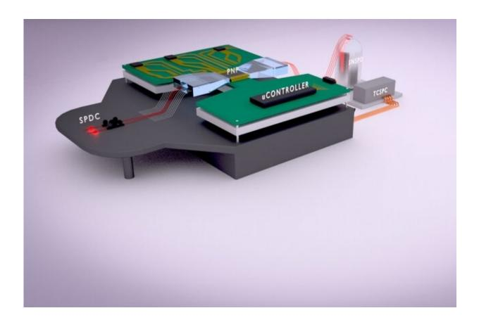
Researchers from MIT, Google, and elsewhere have designed a novel method for verifying when quantum processors have accurately performed complex computations that classical computers can't. They validate their method on a custom system (pictured) that's able to capture how accurately a photonic chip ("PNP") computed a notoriously difficult quantum problem. Credit: Mihika Prabhu
