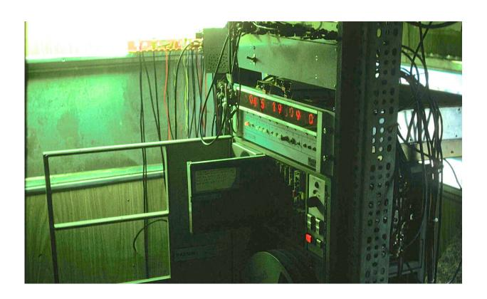
14-track recorder used to record the telemetered data from the 1980 Mount St. Helens pre-eruption seismic sequence. Credit: Stephen Malone
