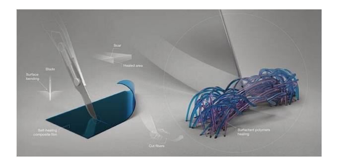
The mechanical and thermoelectrical self-healing process of the composite film.Reproduced with permission from reference one. Credit: WILEY-VCH Verlag GmbH
