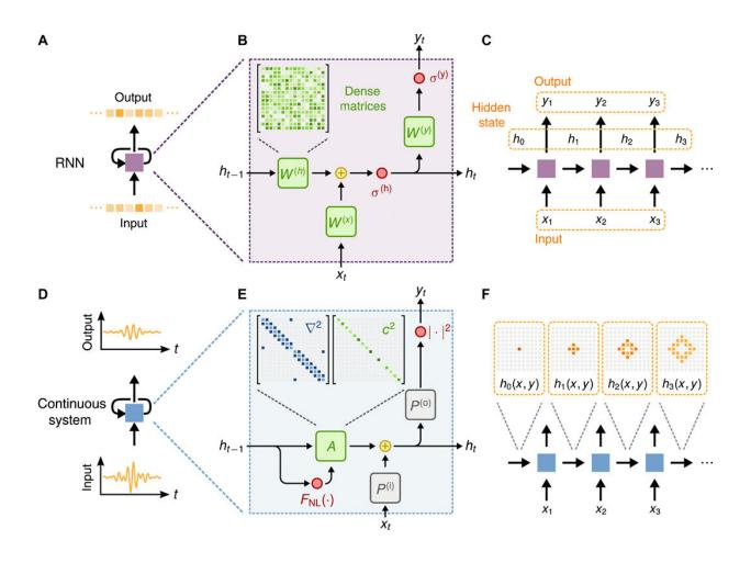
Conceptual comparison of a standard RNN and a wave-based physical system. (A) Diagram of an RNN cell operating on a discrete input sequence and producing a discrete output sequence. (B) Internal components of the RNN cell, consisting of trainable dense matrices W(h), W(x), and W(y). Activation functions for the hidden state and output are represented by  $\sigma(h)$  and  $\sigma(y)$ , respectively. (C) Diagram of the directed graph of the RNN cell. (D) Diagram of
