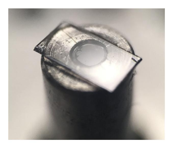
Spinning diamond. A small slab of diamond is mounted on a motor shaft that can rotate at 200,000 rpm. Probing a single quantum spin within the crystal revealed the influence of the rotation on the spin. Credit: A. Wood/Univ. of Melbourne
