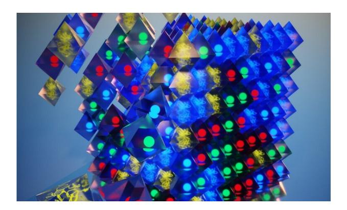
A schematic of the programmable assembly of 3-D ordered nanostructures from material voxels that can carry inorganic or organic nanoparticles with different functions, such as light emitters and absorbers, proteins, and enzymes with chemical activity. Material voxels are fabricated from DNA and nano-objects of different kinds, and their assembly is guided by the voxel design and DNA-programmable interactions. Credit: Brookhaven National Laboratory
