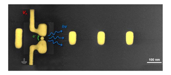
Let there be light - and it was directional: The world's first electrically powered Yagi-Uda antenna was built at the University of Würzburg's Department of Physics. Credit: Department of Physics / JMU
