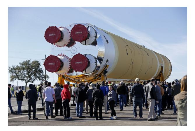
Employees and contractors watch as the core stage of NASA's Space Launch System rocket, that will be used for the Artemis 1 Mission, is moved to the Pegasus barge, at the NASA Michoud Assembly Facility where it was built, in New Orleans, Wednesday, Jan. 8, 2020. It will be transported to NASA's Stennis Space Center in Mississippi for its green run test. (AP Photo/Gerald Herbert)
