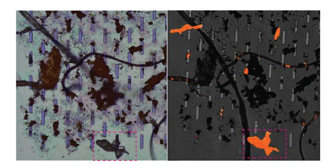
The image at left shows debris captured on a silicon nanomembrane (greenish background, with bluish slots, 8 microns wide) by Greg Madejski in the lab of James McGrath. The fluorescence image at right shows how Nile red stain is used to identify the plastics. Credit: McGrath lab
