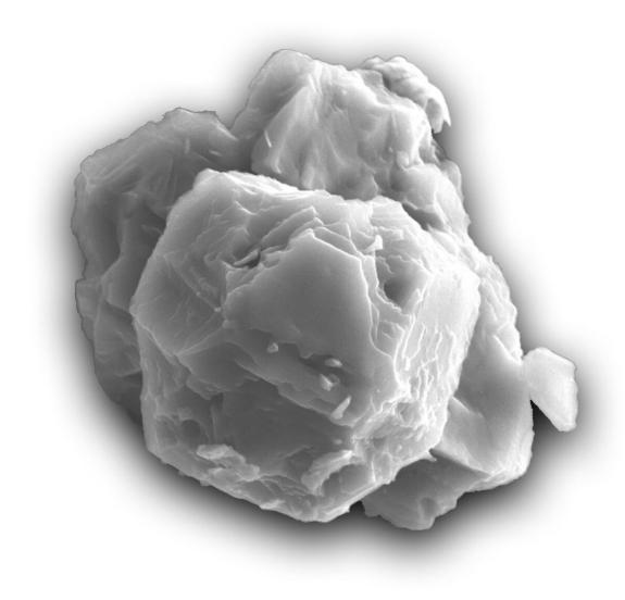
Scanning electron micrograph of a dated presolar silicon carbide grain. The grain is ~8 micrometers in its longest dimension. Credit: Janaína N. Ávila.
