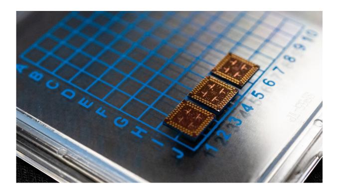
ORNL-developed cryogenic memory cell circuit designs fabricated onto these small chips by SeeQC, a superconducting technology company, successfully demonstrated read, write and reset memory functions. Credit: Carlos Jones/Oak Ridge National Laboratory, U.S. Dept. of Energy
