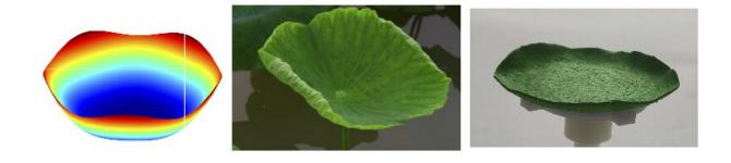
Math imitates life. The new model allows different leaf layers to grow at different rates, a necessary component to generate the bending needed for a bowl-shaped lotus leaf, shown here as the model prediction (left), as seen in nature (middle), and as it appeared in experiments with a leaf-imitating rubber (right). Credit: F. Xu et al., Phys. Rev. Lett. (2020)
