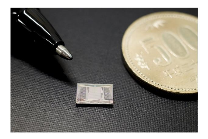
A small-sized silicon photonics chip that can be used for non-mechanical beam steering and scanning. Credit: Yokohama National University
