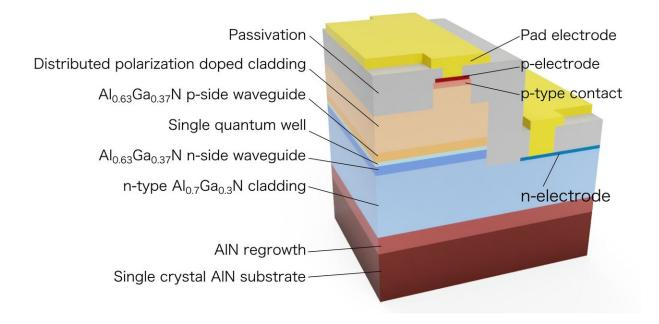
Cross-sectional structure of the UV-C semiconductor laser diode. Credit: 2019 Asahi Kasei Corp. and Nagoya University
