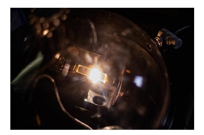
Carbon black powder turns into graphene in a burst of light and heat through a technique developed at Rice University. Flash graphene turns any carbon source into the valuable 2D material in 10 milliseconds. Credit: Jeff Fitlow/Rice University
