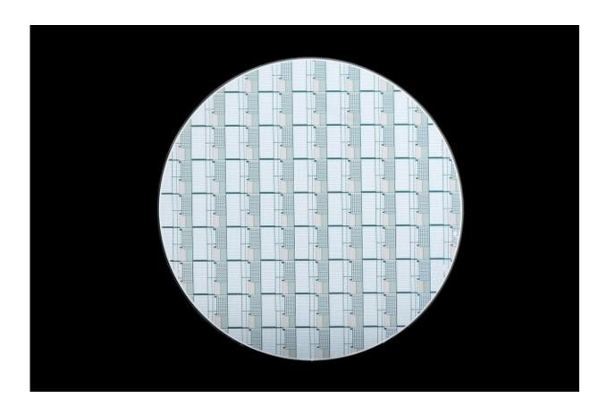
This 8-inch wafer contains phase-change pixels that can be controlled to modulate light. Researchers are studying the properties and behaviors of the pixels to inform the creation of future devices that use phase-change materials. Credit: Nicole Fandel
