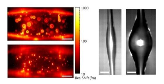
Left: Photothermal maps of a microbubble resonator, both out-of-focus (top), and in-focus (bottom). Scale bars 20µm. Right: Optical micrographs of two microbubble resonators with different geometries. Scale bars 20µm. Credit: ACS Nano; https://pubs.acs.org/doi/abs/10.1021/acsnano.9b04702
