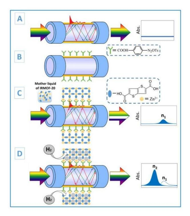
Schematic representation of fabrication and action of present hydrogen sensor design, based on ofplasmon-active optical fiber surface decorated with IRMOF-20 film. Credit: Department of Solid State Engineering, University of Chemistry and Technology, 16628 Prague, Czech RepublicResearch School of Chemistry and Applied Biomedical Sciences, Tomsk Polytechnic University,
