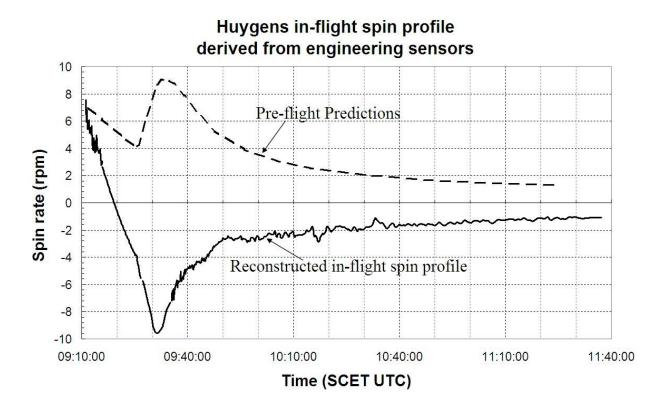
This graph shows the 'spin profile' of ESA's Huygens probe as it descended to the surface of the Saturnian moon Titan on 14 January 2005: the dotted line shows the predicted profile, while the solid line shows the actual profile as tracked by the probe's onboard engineering sensors. The horizontal axis indicates UTC time and the vertical axis the spin rate (in revolutions per minute). Credit: Reproduced from Lebreton et al. (2005)
