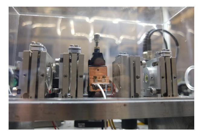
Image showing the source of squeezed light in the experiment (i.e., an optical parametric oscillator). Credit: Jonas S. Neergaard-Nielsen.
