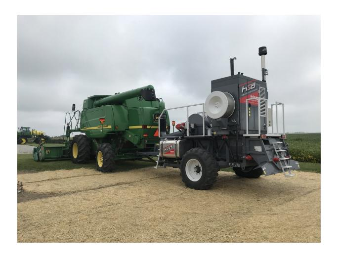
A new University of Illinois study tested the weed-seed-killing power of the Harrington Seed Destructor, an impact mill used to reduce the weed seed bank at harvest. Credit: Lauren Quinn, University of Illinois
