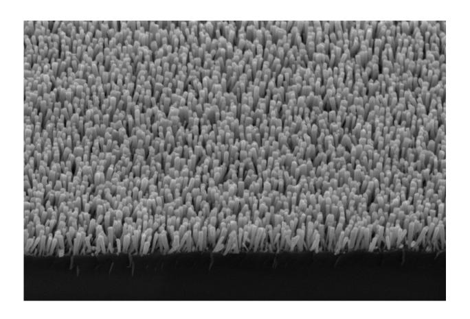
An electron microscope image shows the semiconductor nanowires. These deliver electrons to metal nanoparticles, which turn carbon dioxide and water into methane. Credit: Baowen Zhou
