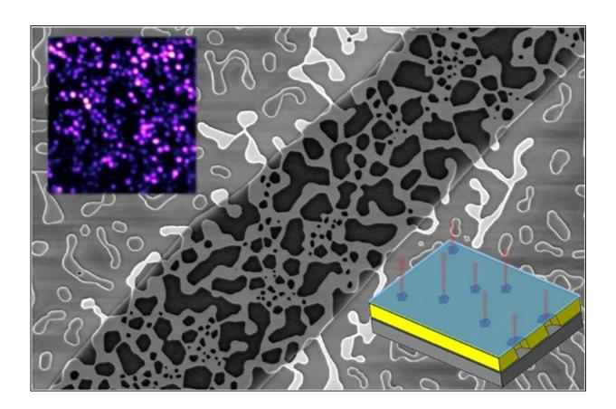
Suspended two-dimensional crystals over pores in a slab of gold (center image) allow NRL scientists to connect quantum light sources (inset images) in a readymade network. Credit: Jeremy Robinson/U.S. Naval Research Laboratory
