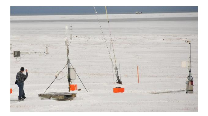
David Cook, a recently retired Argonne meteorologist, performs maintenance on an eddy correlation flux measurement tower, operated by the DOE-funded Atmospheric Radiation Measurement (ARM) program, in Utqiavik, Alaska. The tower exemplifies one of several types of instrumentation used to generate the data in this study. Credit: Argonne National Laboratory/Ryan Sullivan
