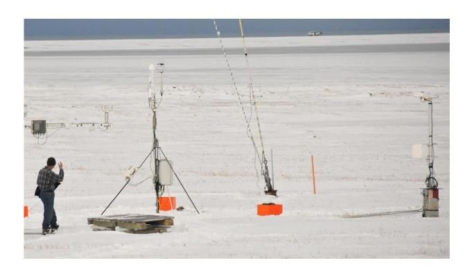
David Cook, a recently retired Argonne meteorologist, performs maintenance on an eddy correlation flux measurement tower, operated by the DOE-funded Atmospheric Radiation Measurement (ARM) program, in Utqiavik, Alaska. The tower exemplifies one of several types of instrumentation used to generate the data in this study. Credit: Argonne National Laboratory/Ryan Sullivan
