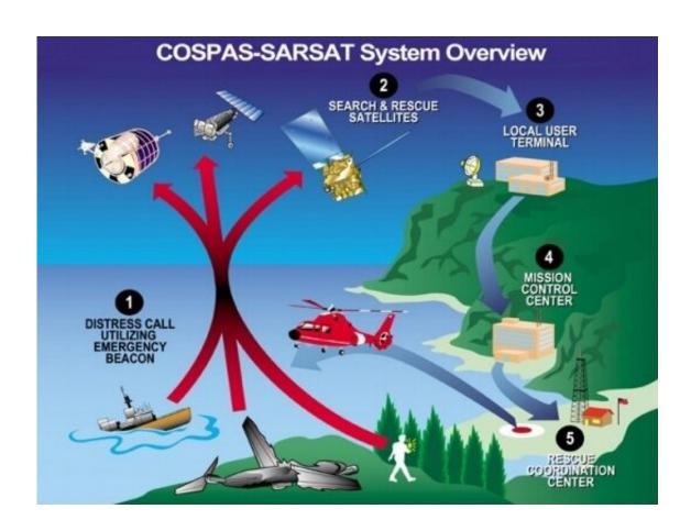
For three decades the Cospas–Sarsat system has used relays on satellites such as Europe's MSG and MetOp to pick up distress calls from ships and aircraft. Credit: Cospas-Sarsat
