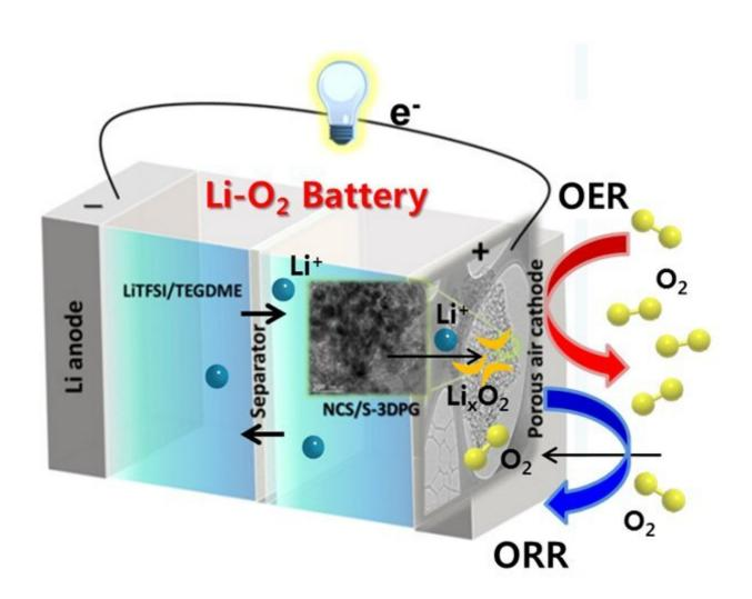
The cathode is designed to facilitate the uptake and release of oxygen, processes that are needed for discharging and charging a lithium-air battery. Credit: DGIST
