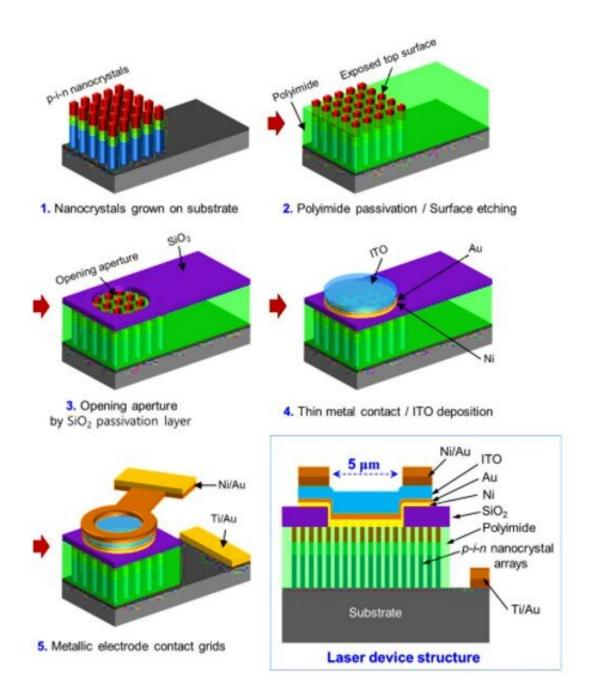
The NCSEL device fabrication. The nanocrystal surface-emitting laser (NCSEL) device was fabricated by the following steps. Schematic illustration of the full device fabrication, including passivation, planarization, photolithography, and contact metallization techniques. Credit: Science Advances, doi: 10.1126/sciadv.aav7523
