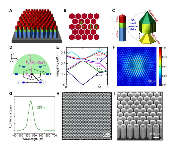
Design of InGaN NCSEL diodes operating in the green wavelength. (A) Schematic of the InGaN nanocrystal arrays for the surface-emitting laser diode. (B) The diameter and lattice constant of the nanocrystals denoted as d and a, respectively. (C) Schematic of the InGaN/AlGaN nanowire heterostructure,
