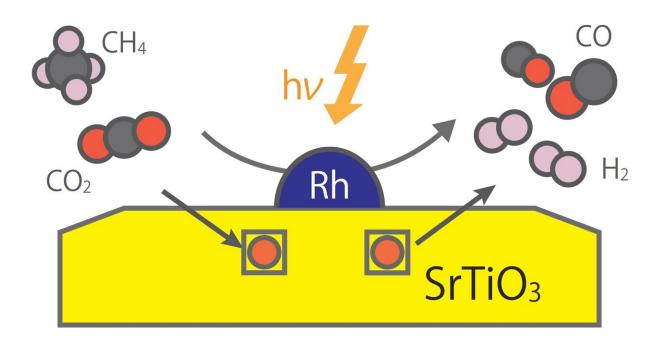
Strontium titanate combined with rhodium nanoparticles converted methane and carbon dioxide into synthesis gas under light irradiation at much lower temperatures that those required in thermal reactors. Credit: Tokyo Tech
