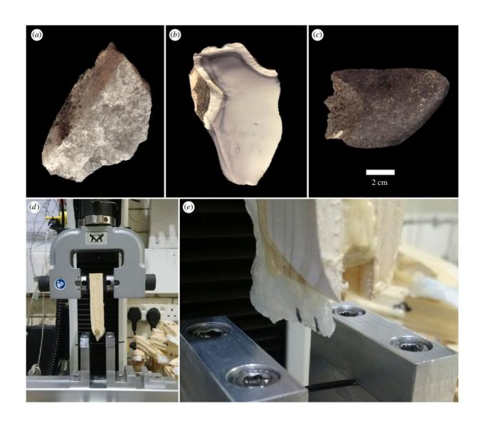
Representative flakes made from quartzite (a), chert (b) and basalt (c). The Instron 3345 tensile testing machine used during the controlled cutting tests (d). A quartzite flake, prior to being used to cut, is clearly depicted, along with the
