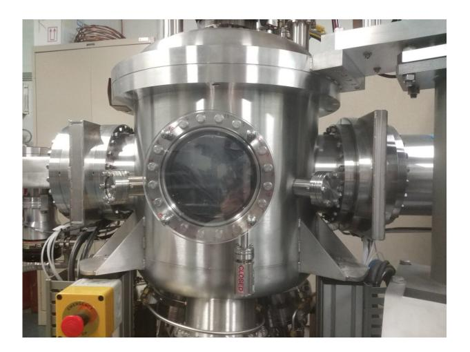
Magnetron-sputtering based plasma reactor used for the preparation of the photoelectrodes of titanium oxide co-doped with nitrogen and tungsten. Credit: My Ali El Khakani, INRS
