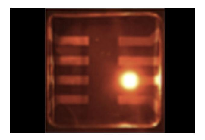
Colloidal quantum dots operating in LED mode. Credit: Los Alamos National Laboratory
