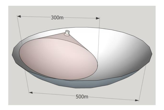
FAST has a 500 meter diameter but only 300 meters is "illuminated" at once. Image Credit: By Phoenix7777—Own workData source: (2011-05-20). "The Five-Hundred-Meter Aperture Spherical Radio Telescope (FAST) Project" Credit: International Journal of Modern Physics D 20 (6): 989–1024. DOI:10.1142/S0218271811019335., CC BY-SA 4.0, https://commons.wikimedia.org/w/index.php?curid=51795209
