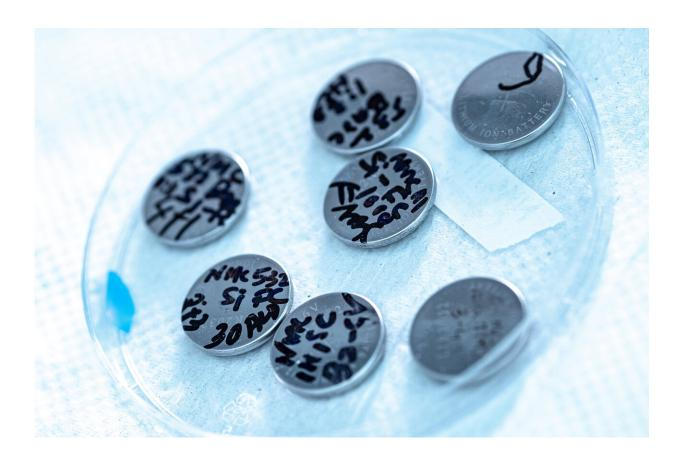
Rice University engineers built full lithium-ion batteries with silicon anodes and an alumina layer to protect cathodes from degrading. By limiting their energy density, the batteries promise excellent stability for transportation and grid storage use. Credit: Jeff Fitlow/Rice University
