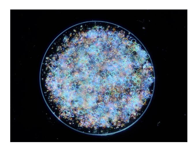
Darkfield microscopy image of a single multi-compartmentalized capsule containing thousands of catalytic protocells that decompose hydrogen peroxide into water and oxygen gas. Credit: Dr. Pierangelo Gobbo and Dr. B. Pavan Kumar, University of Bristol
