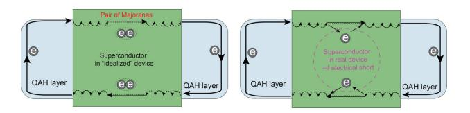
An exotic quantum state known as a "chiral Majorana fermion" is predicted in devices wherein a superconductor is affixed on top of a quantum anomalous Hall (QAH) insulator (left panel). Experiments performed at Penn State and the University of Würzburg in Germany show that the millimeter-size superconductor strip used in the proposed device geometry creates an electrical short, preventing the detection of chiral Majoranas (right panel). Credit: Cui-zu Chang, Penn State
