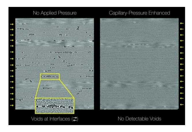
MIT researchers have devised a way to manufacture autoclave-formulated aerospace-grade advanced carbon fiber composites without utilizing applied pressure from an autoclave. Cross-sections of the composites show that a nanoporous film with morphology-controlled nanoscale capillaries provides the needed pressure at the interfaces in layered polymeric architectures. Credit: Massachusetts Institute of Technology
