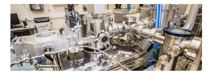
An atomic layer deposition reactor used for obtaining ultrathin molybdenum oxide films, which were subsequently sulfurized to 2D molybdenum disulfide. Credit: Atomic Layer Deposition Lab, MIPT
