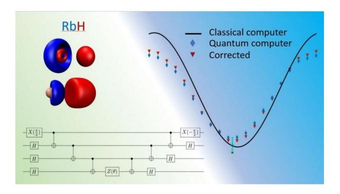
An ORNL research team lead is developing a universal benchmark for the accuracy and performance of quantum computers based on quantum chemistry simulations. The benchmark will help the community evaluate and develop new quantum processors. (Below left: schematic of one of quantum circuits used to test the RbH molecule. Top left: molecular orbitals used. Top right: actual results obtained using the bottom left circuit for RbH). Credit: Oak Ridge National Laboratory
