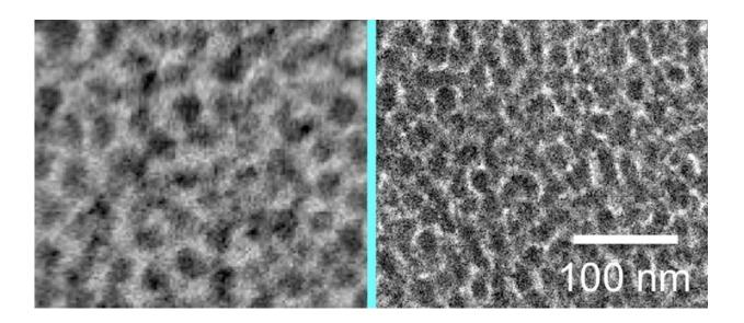
TESET, before and after water treatment. The water has changed the structure in the material. Credit: Kenneth P. Mineart, NCSU
