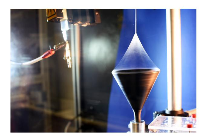
Electrospinning of a multifibrillar polyacrylonitrile fiber. Credit: University of Bayreuth / Rennecke.
