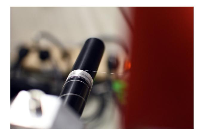
Stretching of a multifibrillar polyacrylonitrile fiber. Credit: University of Bayreuth / Rennecke.
