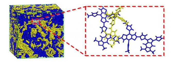
Organic photovoltaic material has two molecular components, shown here in blue and yellow. The blue molecule is an electron donor, and the yellow molecule is a non-fullerene (electron) acceptor (NFA). Modeling in a new study has shown that a minuscule tweak to the NFA drastically raises the rate of conversion of light into electricity. Credit: Georgia Tech/Bredas lab/Tonghui Wang
