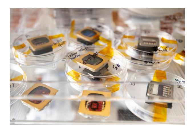
Selection of solar cells in the laboratory of GTRI Principal Research Engineer Jud Ready. The cells include 3D, CZTS, organic photovoltaic, and silicon. Credit: Georgia Tech/Branden Camp
