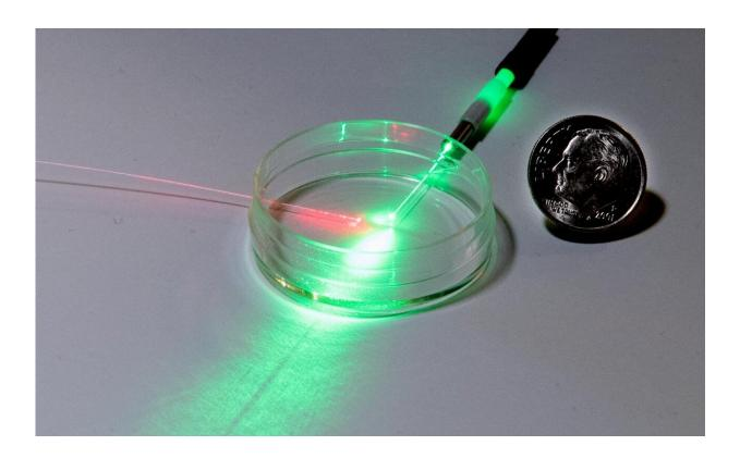
An empty petri dish with two optical fibers, illustrating one version of the researchers' experiment. The left-hand fiber (usually shining infrared light, but depicted here as visible red light) is a temperature sensor. The top fiber shines green, red or blue light into the petri dish to adjust the signal that the temperature sensor measures. Credit: J.L. Lee/NIST
