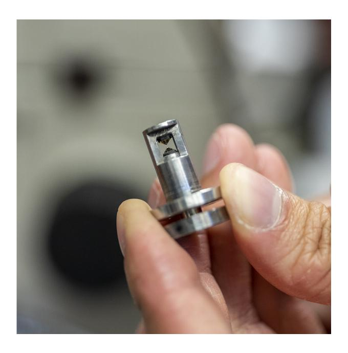
A diamond anvil cell. By compressing a sample between these two opposing anvils, pressures greater than the center of the Earth can be achieved. Credit:
